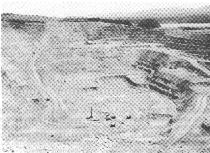
PHOTO 6 - Open pit, Island Copper Mine, currently operating at 40 000 tonnes per day. Initial reserves 257 million tonnes grading 0.52 percent Cu, 0.017 percent Mo, plus precious metal and rhodium credits
