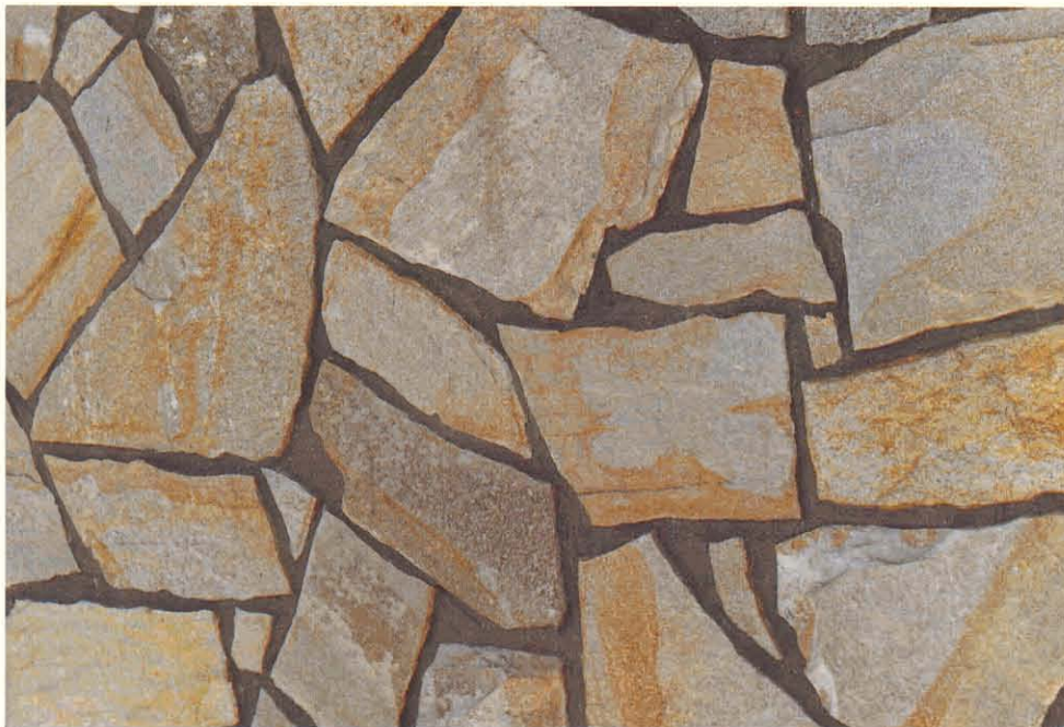
Flagstone produced from a quarry near Revelstoke (micaschist) is used as a decorative stone.
