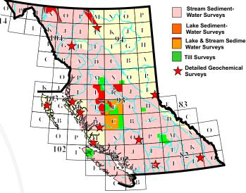
Results of sampling at a density higher than 1:250 000 reconnaissance scale stream sediment and water surveys or using other media such as lake sediment add value to the RGS database. These surveys are applied to areas where conventional stream sediment sampling is unsuitable or to focus on a specific target. Survey sample types for which data has been published include lake sediment, till and heavy mineral concentrate.
