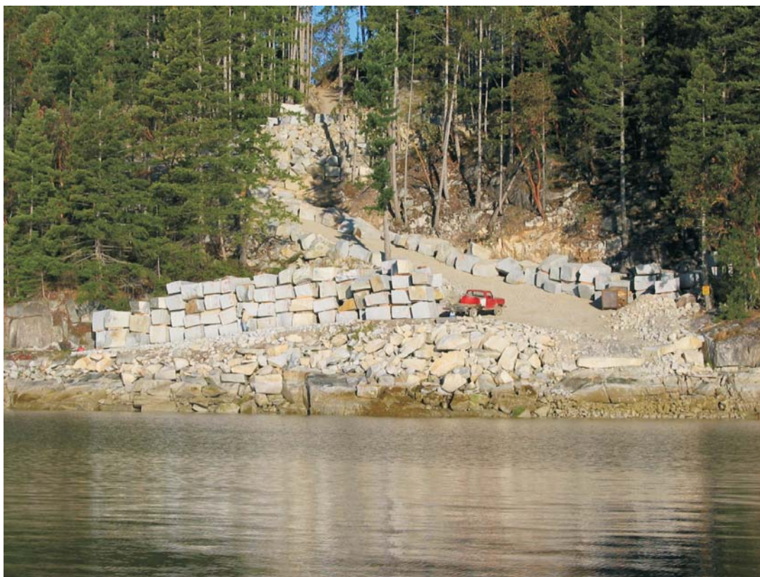
Figure 9. Hardy Island Granite (granodiorite) - blocks ready for shipping (flat bed truck for scale).
