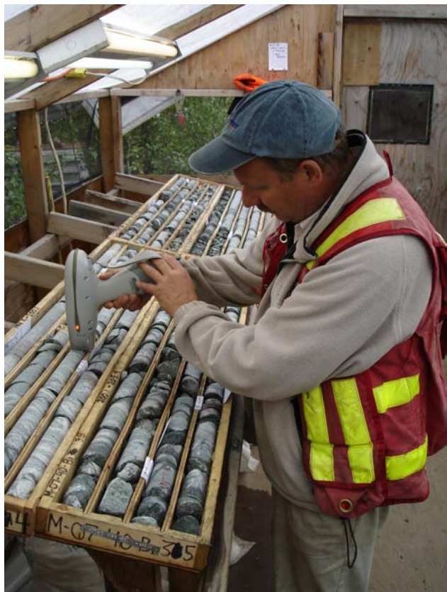
Photo 14. Portable XRF analyzer gives immediate indication of copper, and by inference the gold grade of Mitchell zone drill core.
