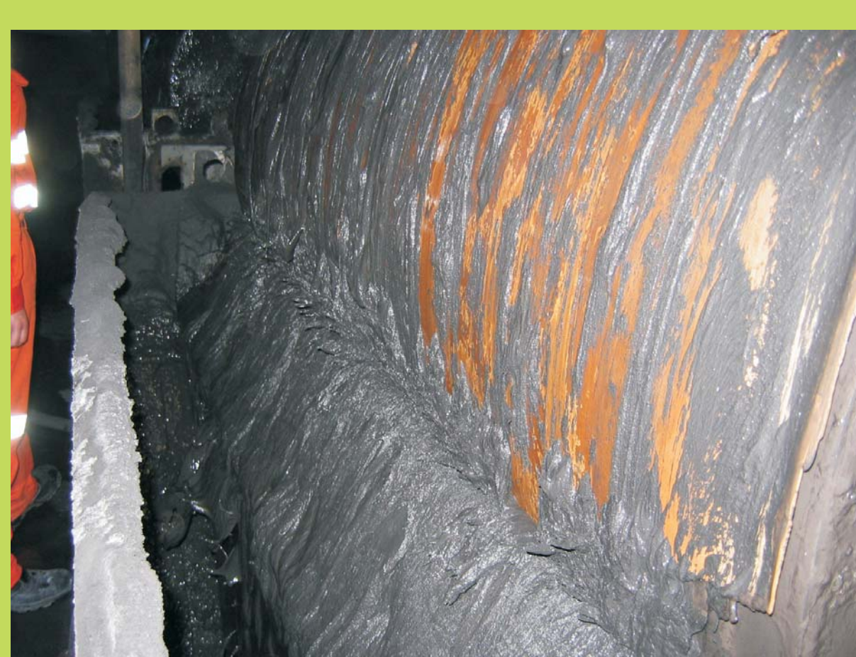
Fig. 4c Magnetite is recovered by magnetic separation and recycled.
