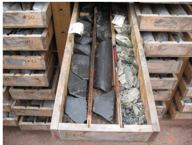
Photo 27. Massive magnetite at the Brynnor project. Brynnor is a 1960s past-producer of iron ore, one of several magnetite skarns on the coast that are subject to re-examination in light of recent demand for iron ore.
