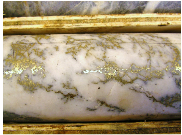
Photo 12. Brucejack bonanza gold, 0.6 m grading 18 755 g/t Au and 9312 g/t Ag from 60.60 m in drillhole SU-115. Photo courtesy of Pretium Resources.
