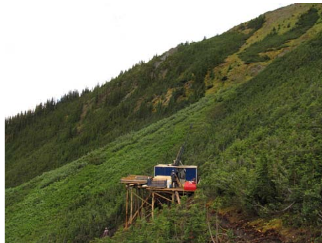
Photo 19. Diamond drilling on the Northwest extension of the Akie SEDEX project (courtesy Canada Zinc Metals).
