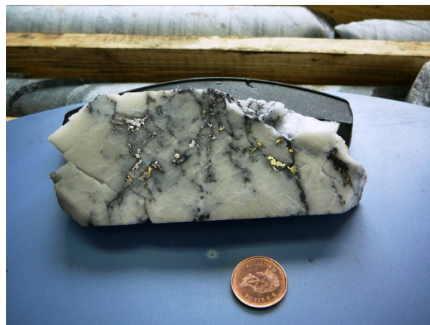
Photo 16. A remarkable drill intersection outside of the proposed pit limits at the Cariboo Gold Quartz project of Barkerville Gold Mines Ltd. Hole CM11-25B intersected 19.9 m of 83 g/t Au (not true width) of gold-cosalite-pyrite-quartz mineralization.
