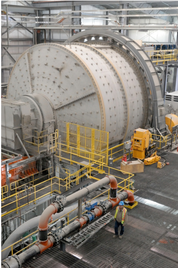
Photo 3. New 30 000 tonne/day mill at Copper Mountain (courtesy Copper Mountain Mining Corporation).
