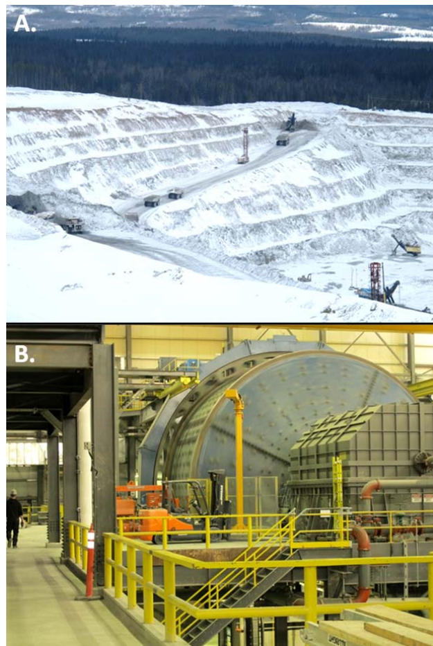
Photo 4. Operations at the Endako molybdenum mine. Photo A. Mining in the West Denak pit to supply a low-grade stockpile; Photo B. New Semi-Autogenous Grinding (SAG) mill.
