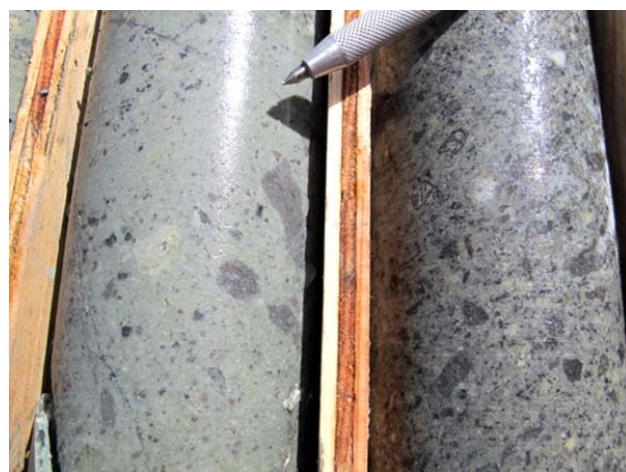
Photos 17. The exploration program at the Blackwater gold-silver project was the biggest in the province and included resource and geotechnical drilling of about 236 606 metres. Vqr "Photo. Vj g" delineation drilling grid from above (Photo by Lori Borth); Bottom Photo. Bleached versus less altered lapilli tuff with garnet replacement of fragment.
