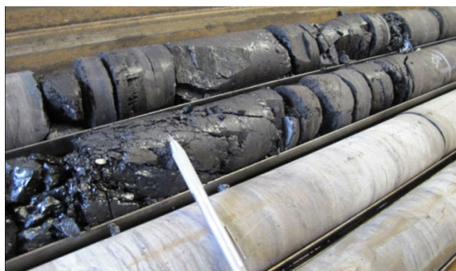
Figure 7: Gething Formation coal seam No. 31 in core, Cardero Coal's Carbon Creek project.
