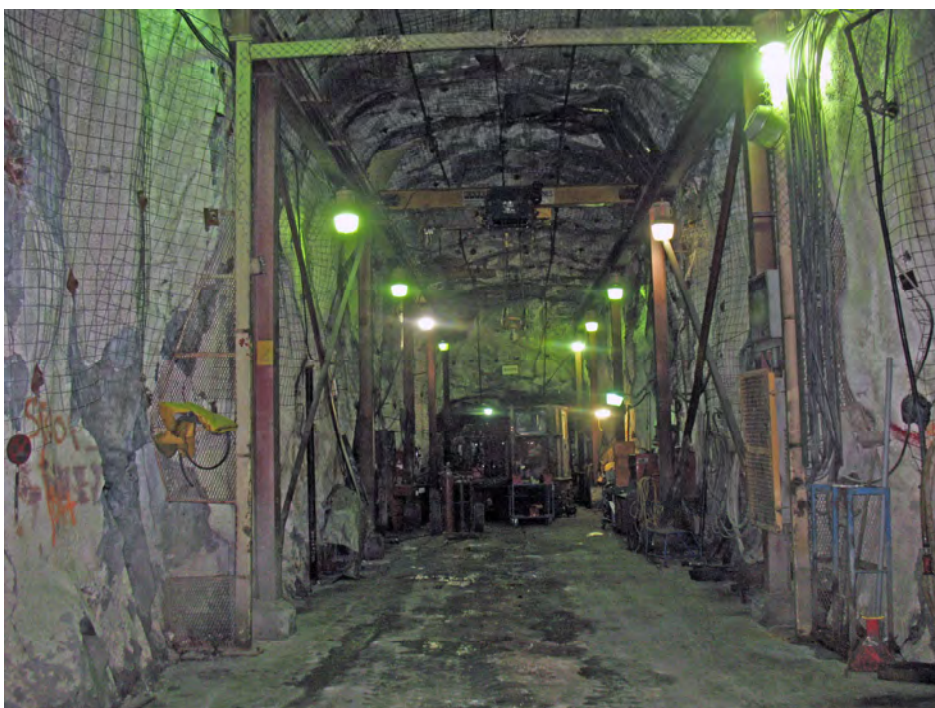
The province's producing polymetallic mine is the Myra Falls operation on Vancouver Island. With limited surface availability, mining equipment is assembled and maintained in underground workshops such as this.
