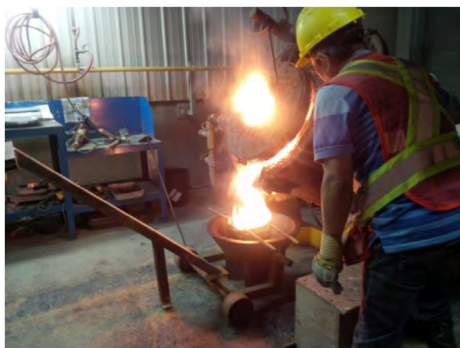
Fig. 3. Bonanza Ledge, first gold pour in July, 2014. Courtesy of Barkerville Gold Mines Ltd.
