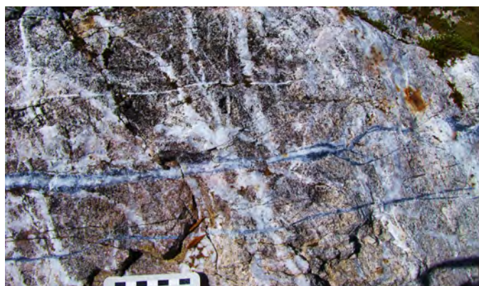
Fig. 23. Sheeted quartz-molybdenite veins cutting Lime Creek intrusive complex quartz monzodiorite at Kitsault.
