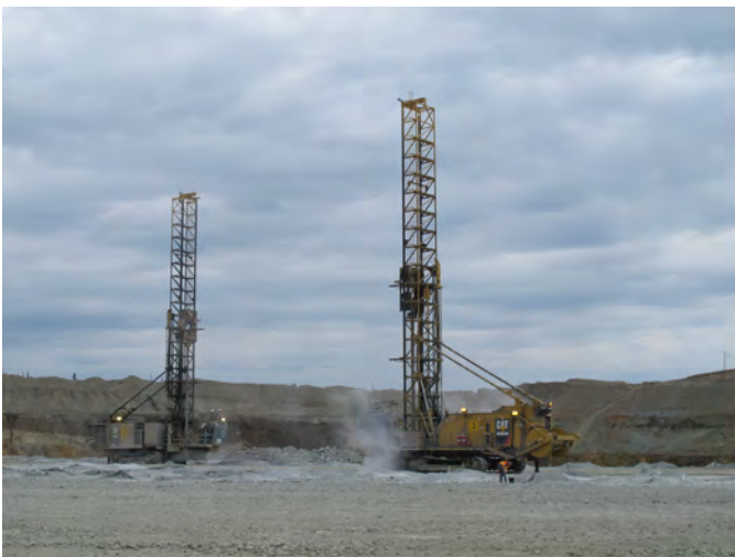
Fig. 8. Blast-hole drilling for Phase 2 mining in the MBX pit, Mt. Milligan mine.
