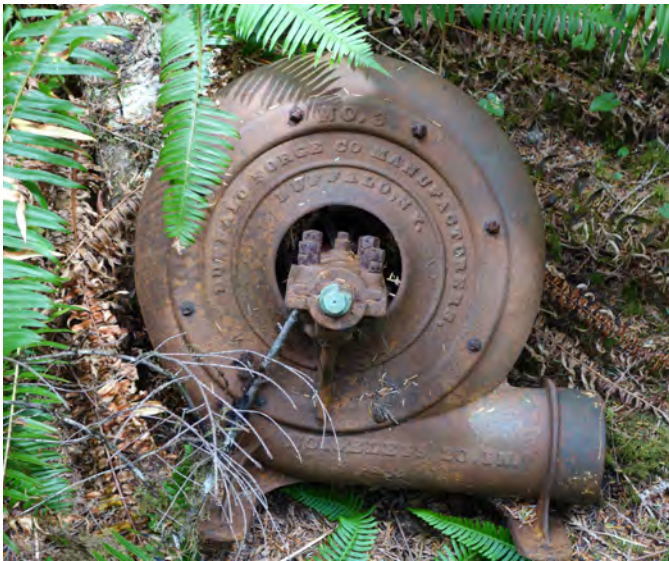
Fig. 13. A forge blower at abandoned workings on the Pacific Iron property, probably dating to 1916.
