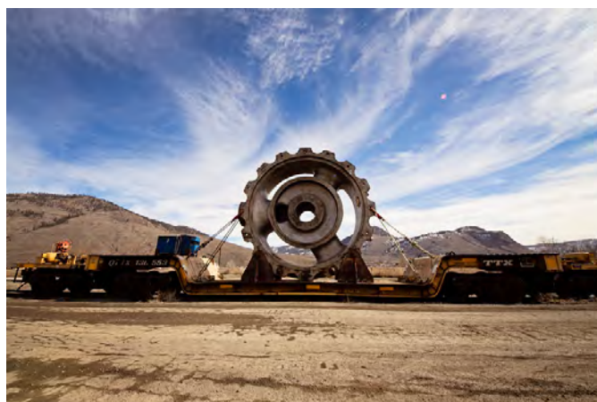
Fig. 4. Parts for new secondary crusher on the way to Copper Mountain mine. Photo courtesy of Copper Mountain Mining Corporation.
