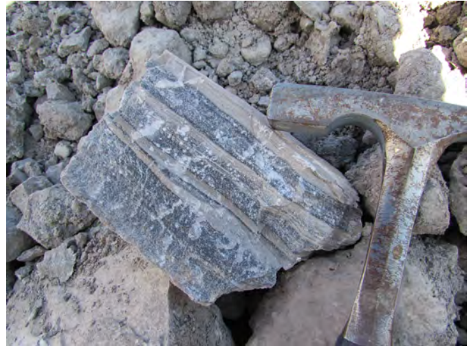
Fig. 18. Laminated evaporitic gypsum, Burnais Formation, Elkhorn mine.
