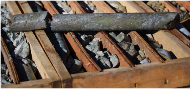
Fig. 13. Chalcopryite-bearing drill core from Teuton Resources Del Norte project. Photo courtesy of Teuton Resources.
