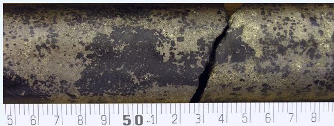
Turnagain: magmatic pyrrhotite with interstitial pentlandite hosted in serpentinized wehrlite (Image courtesy of Hard Creek Nickel Corporation)
