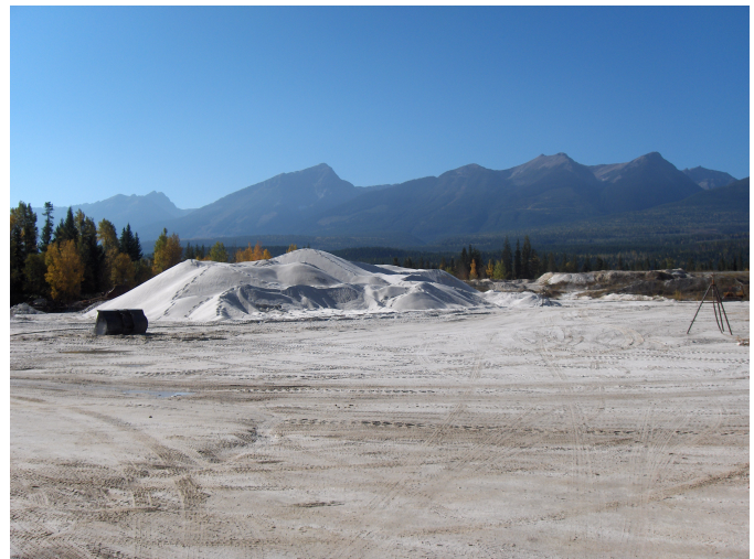
Fig. 15. Stockpiled silica sand at the Moberly Silica mine, which produces silica for glass-making, and other industrial uses. Heemskirk Canada Limited is currently re-developing operations for production of 20 to 140-mesh frac sand for the oil and gas industry.
