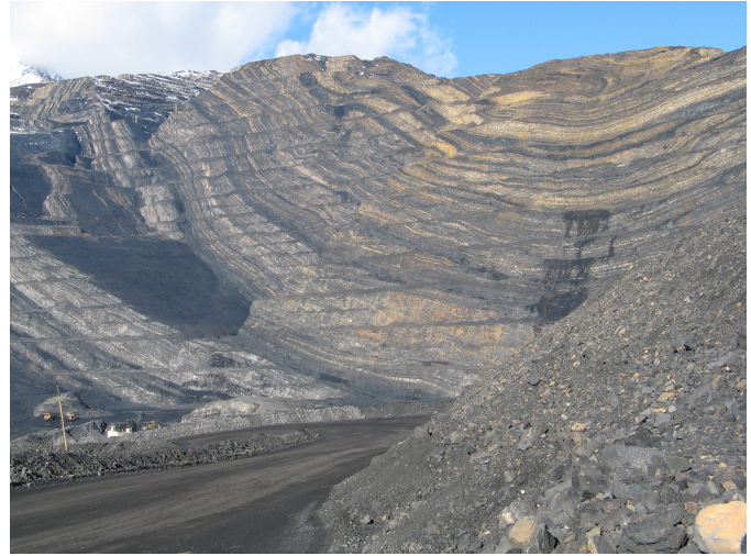
Fig. 13. Coal seams in the Alexander Creek syncline at the Line Creek mine. Photo courtesy of Teck Coal Ltd.
