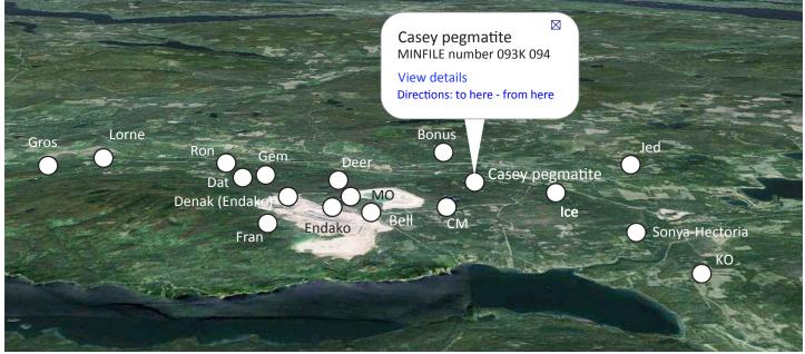
MapPlace queries MINFILE database, displays results on oblique aerial photograph, and links back to database.
