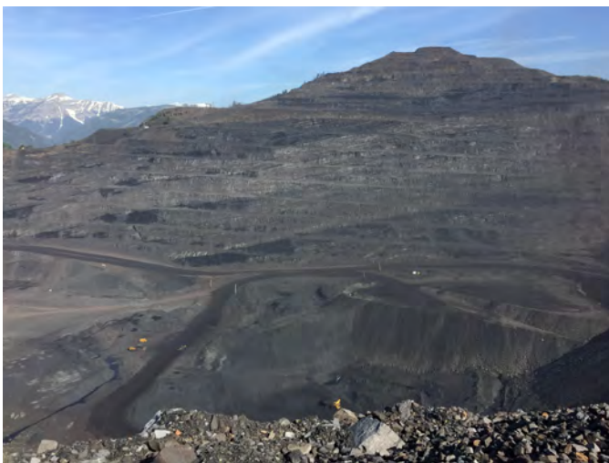
Fig. 6. Dipping Mist Mountain Formation coal seams at the Elkview mine.
