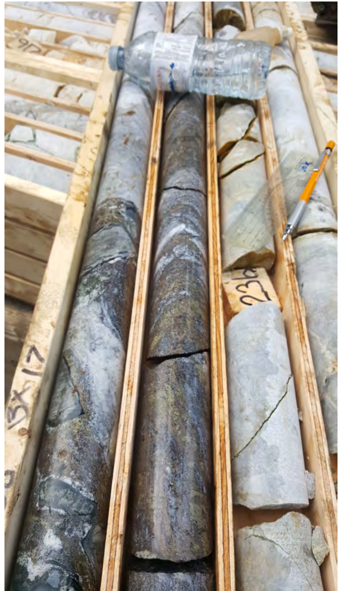
Fig. 17. Zinc-lead mineralized drill core from the Jackpot property. Photo courtesy of Margaux Resources Ltd.
