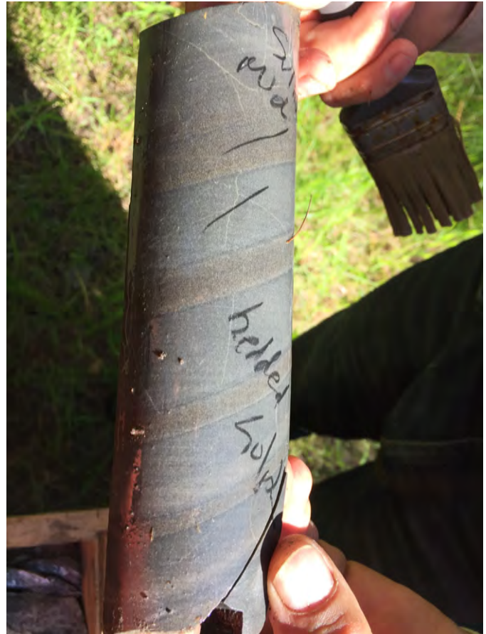
Fig. 14. Bedded sulphides in drill core on the Monroe property.
