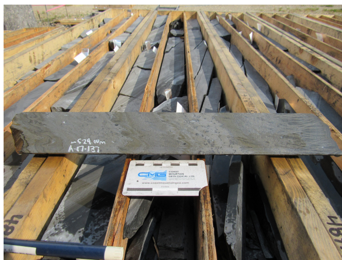
Fig. 9. Mottled high-grade sphalerite and galena, hole A-17-137, at approximately 529 m depth (courtesy of Canada Zinc Metals Corp.).
