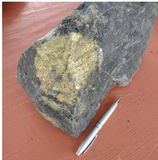
Fig. 2. Ore specimen from Phase 3, Mt. Milligan mine, chalcopyrite and pyrite.
