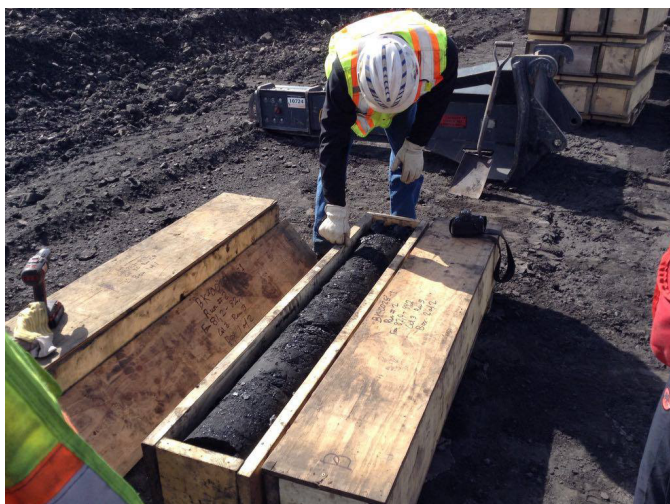
Fig. 9. Large diameter core drilling for coking coal quality testing at the Fording River Swift expansion area.
