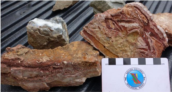
Fig. 4. Epithermal textures (crustiform quartz, chalcedony veining) in hand specimens collected in Talisker Resources Ltd.'s regional exploration of the Spences Bridge belt.
