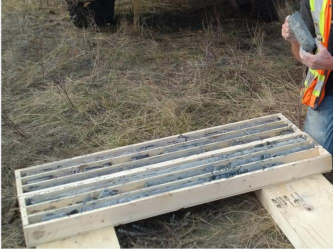
**Fig. 5.** Bentonite clay in drill core at the Mont bentonite prospect. Photo courtesy of L. Lindinger.
