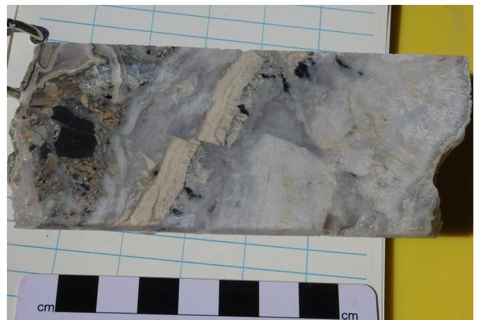
**Fig. 2.** Quartz, chalcedony and adularia veining with ginguero (black) in lapilli tuff at Westhaven Ventures Inc.'s Shovelnose project.
