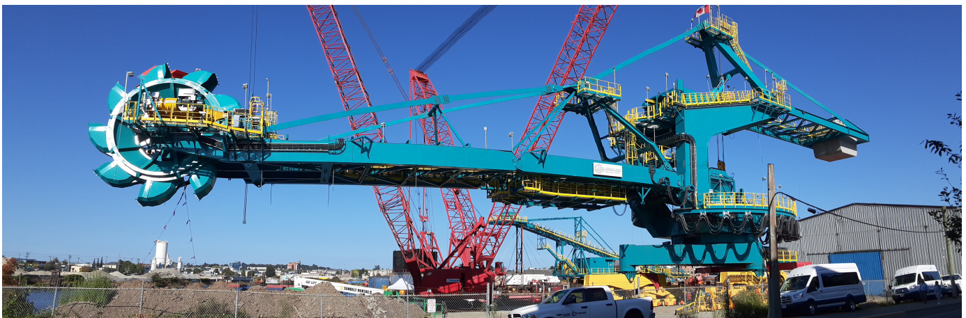
Fig. 10. New coal stacker-reclaimer being assembled at the Point Hope Shipyard in Victoria in the summer of 2020.
