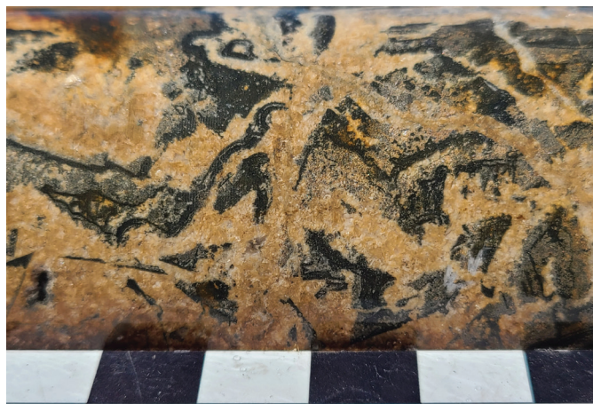
Fig. 6. Barite vein with sulphides and sulphosalts containing gold and silver. Camp Deposit, Silver Queen project (Equity Metals Corporation).
