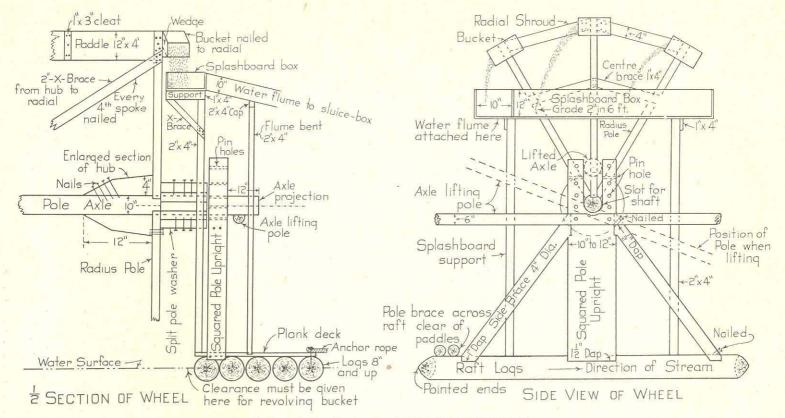
Sections showing Construction of Parts of Undercurrent-wheel.
