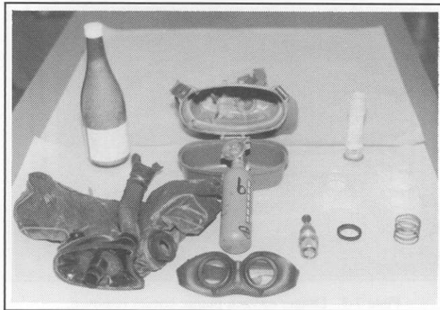
Plate 7-9. Components of Dräger Model OXY-SR 30 self-contained oxygen breathing apparatus.
