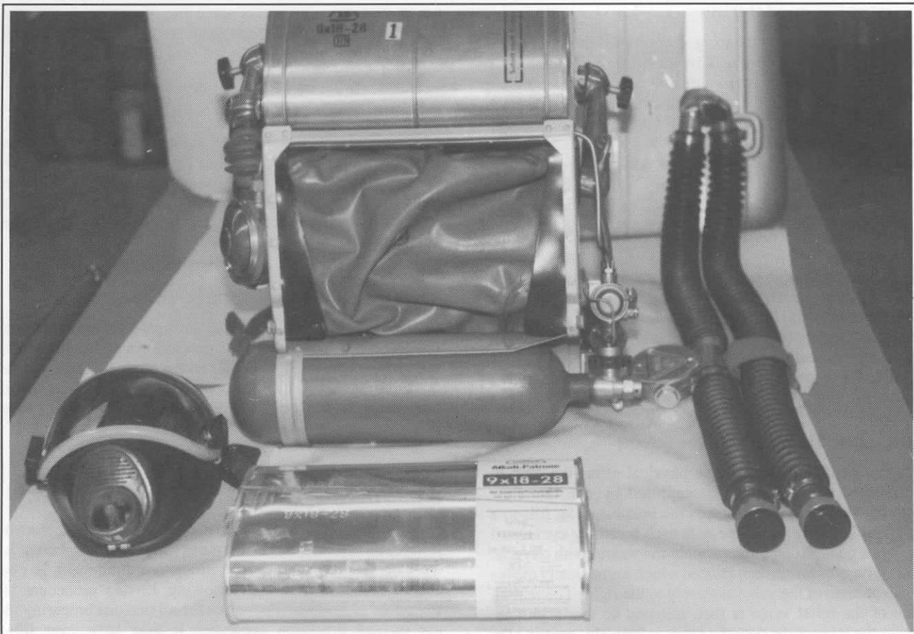
Plate 7-14. Components of Dräger Model BG 174 self-contained breathing apparatus.
