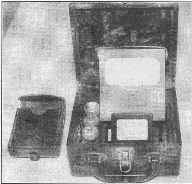
Plate 8-2. A velometer for measuring the rate of flow of air in mine workings.
