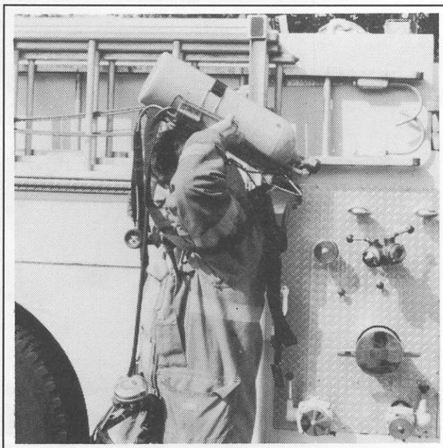
Plate 7-17. Putting on breathing apparatus; the over-the-head method. Step 3: raise the cylinder overhead and let the elbows find the loops in the shoulder harness.
