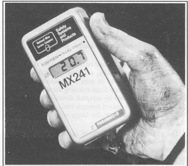
Plate 5-3. NMS MX241 dual sensor gas detector for oxygen and methane.
