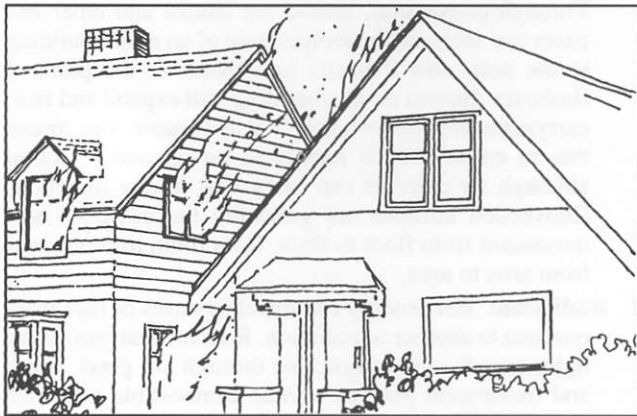
Figure 6-10. Heat transfer by direct contact. Courtesy: Fire Academy — J.I. of B.C.
