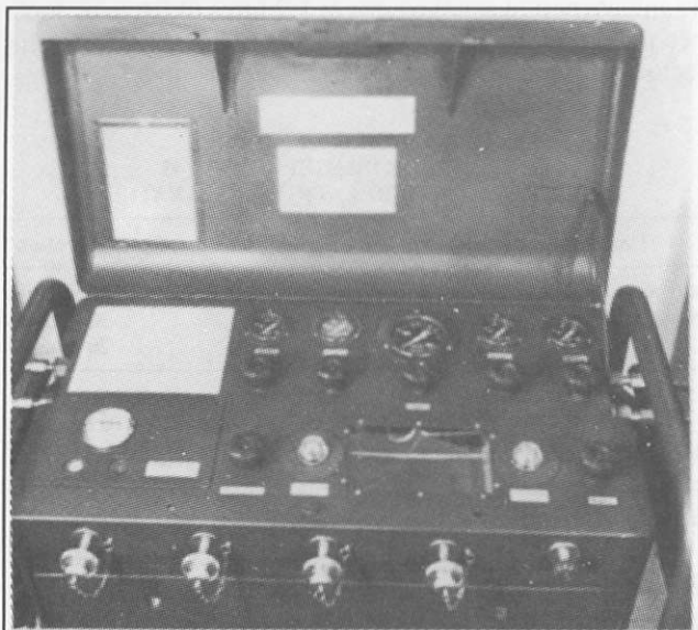
Plate 7-6. Dräger oxygen pump; control panel.
