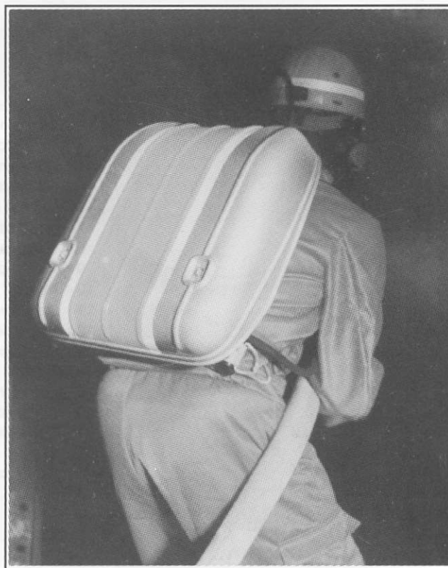
Plate 7-13. Dräger Model BG 174 self-contained breathing apparatus in use.
