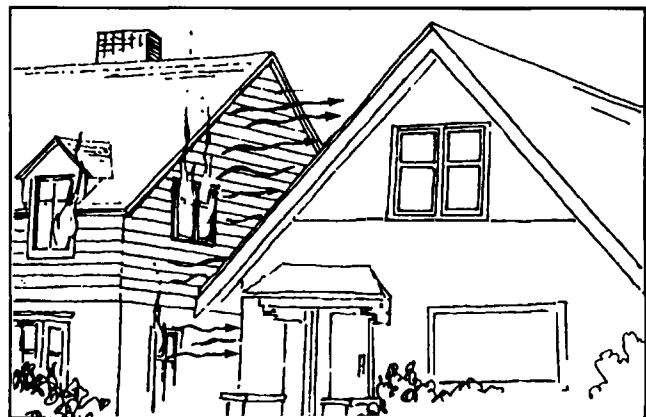
Figure 6-9. Heat transfer by radiation.
