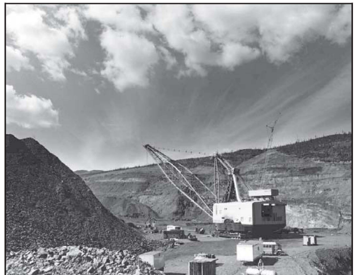
D20. A modern open pit coal mine, the Greenhills mine of Fording Coal Co., showing a Marion walking dragline used for casting off waste-rock overlying the coal. (R.E. Player, AR 1977)
