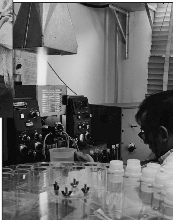
Photo A19. In its third stage of development, starting in the early 1970s, the laboratory depended on instrumental chemistry, principally atomic absorption spectrometry and x-ray fluorescence. Since then it has conducted a complete range of petrochemical and assay analyses and produced them in abundance. Mac Chaudhry is shown operating an atomic absorption spectroscope with an automated sample changer designed in-house by P.F. Ralph in the late 1970s. (R.E. Player, AR 1981)
