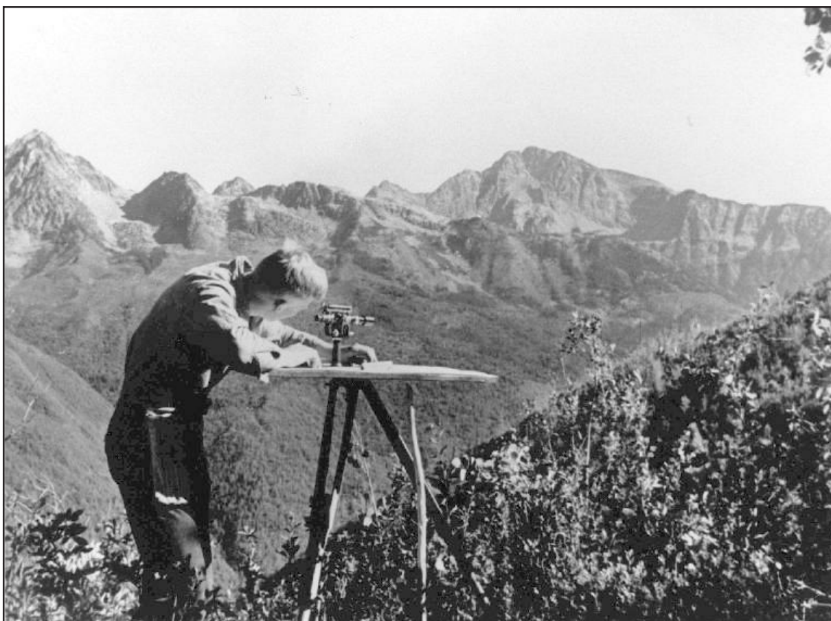
Photo A6. Geological surveying in the Mineralogical Branch period. J.T. Fyles working near Zincton in 1948 sights an alidade on a plane table toward a geological observation point where an assistant holds a stadia rod. With this method topographic and geological maps could be developed at the same time. Relatively large areas were mapped in this manner before the days of abundant aerial photographs and topographic maps. (M.S. Hedley)
