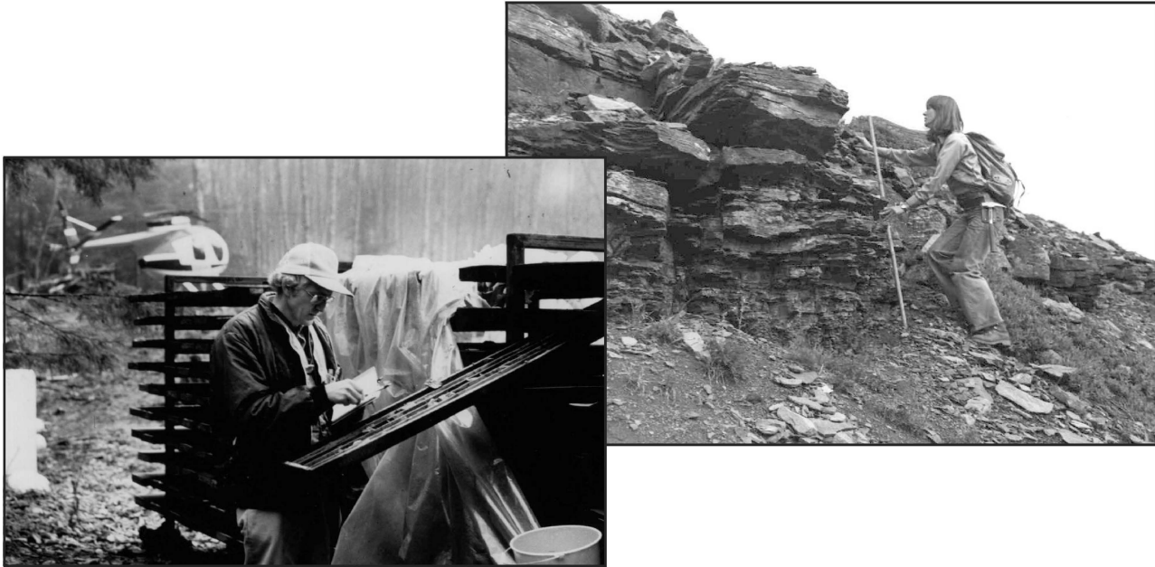
Photo A9. Exploration drilling by industry provides abundant information on the third dimension near prospects. Survey geologists expend much effort examining and logging diamond drill core. Here Bill McMillan is in the unusual situation of logging core while a helicopter waits at a porphyry copper prospect on Gambier Island in 1982.
