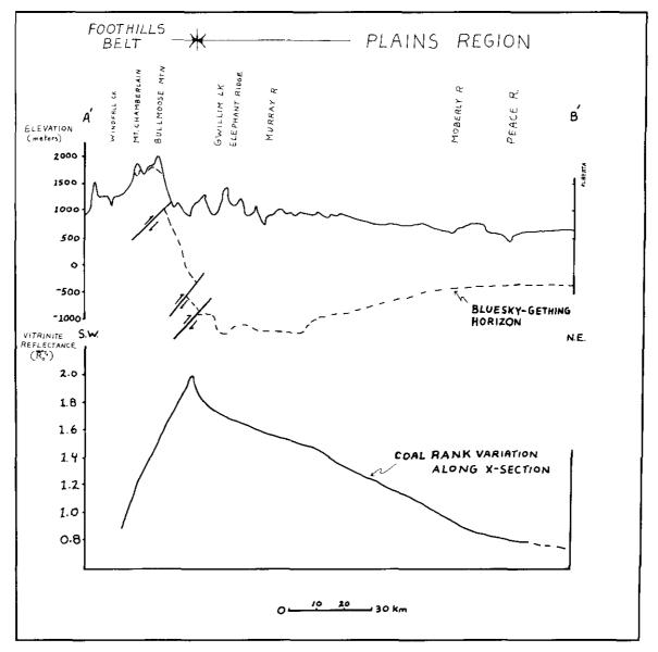
Figure 34. Coal rank variation along cross-section.
