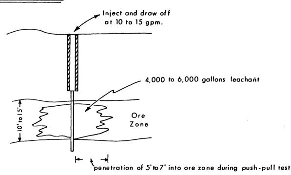
Using these approximate diamensions, this method should sample leach 75 to 125 tons of material. A minimum of 3 wells should be leach tested.
