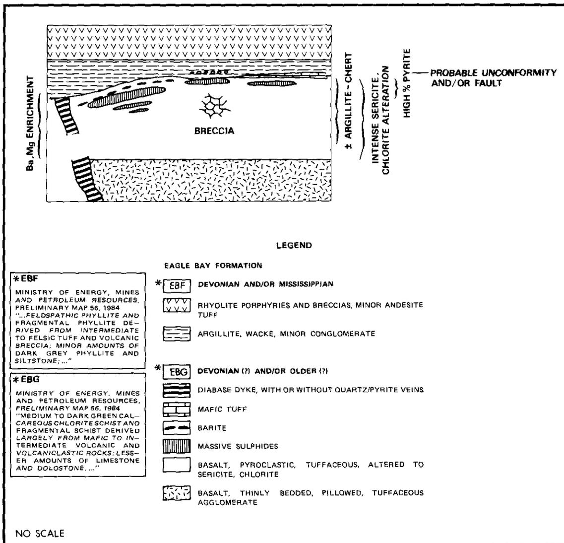
Figure 20. Diagrammatic vertical southeast-northwest section, Hilton-Rea-Falconbridge area.
