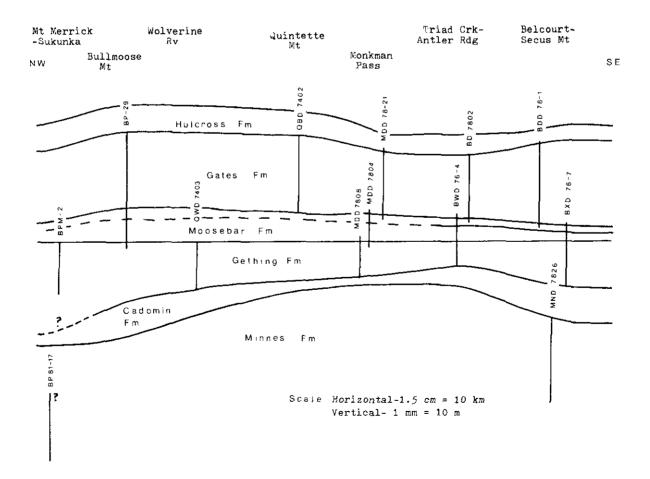
Figure 49-3. Generalized section from Burnt River to Narraway River showing diamond-drill hole sample distribution.
