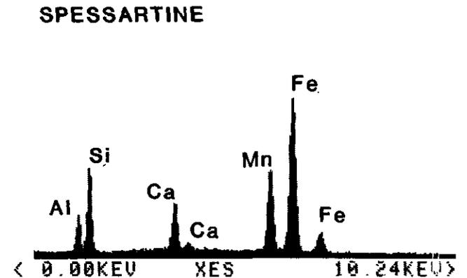
Figure 2-7-4A, B, C, D. Scanning electron microscope analyses of garnets defining the elemental constituents and relative amounts of elements present. Figure 2-7-4A is an almandine garnet  $[\text{Fe}_3\text{Al}_2(\text{SiO}_4)_3]$  from the footwall. Figures 2-7-4B and 2-7-4C (sulphide zone), and 2-7-4D (hangingwall) are spessartine garnets  $[\text{Mn}_3\text{Al}_2(\text{SiO}_4)_3]$ .
