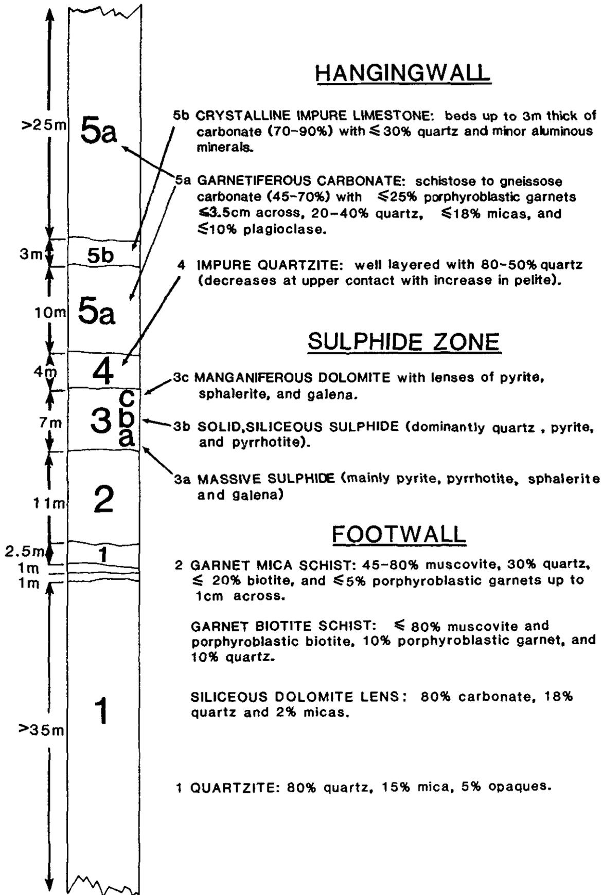
Figure 2-7-2. Detailed stratigraphic column of the 100-metre section studied in the Cummins River canyon. Unit numbers correspond to those in Figures 2-7-2 and 2-7-3.
