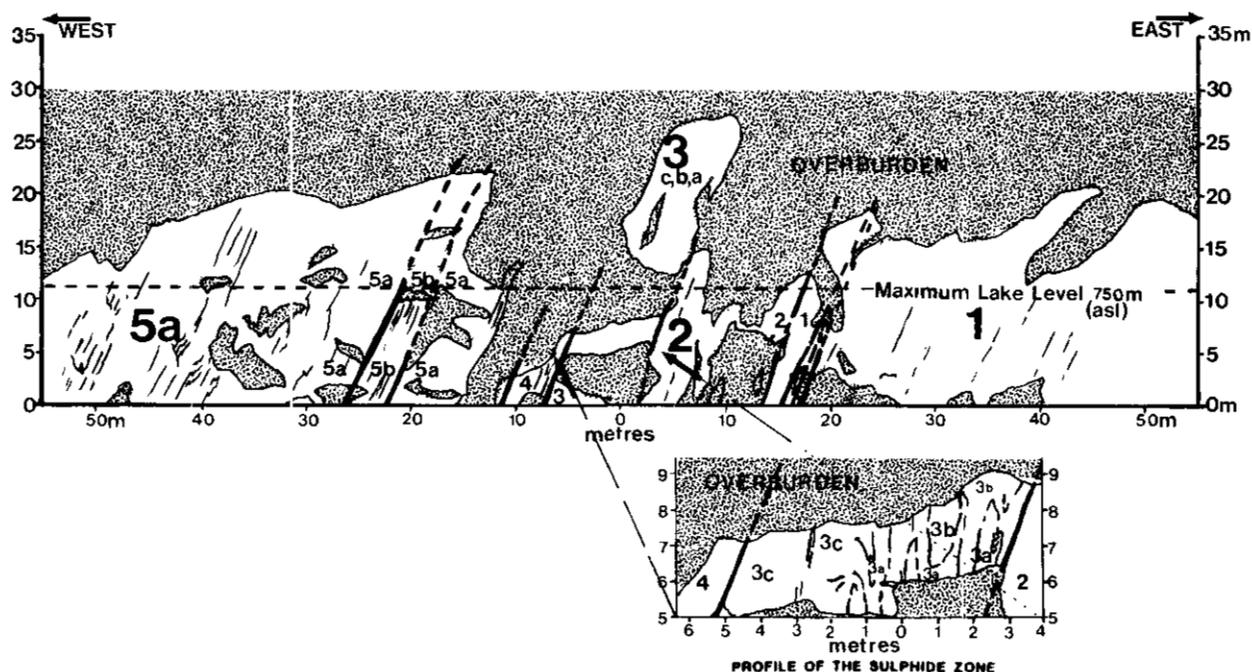
Figure 2-7-3. Profile of the Bend occurrence, Cummins River canyon. Zero on the vertical scale is the level of McNaughton Lake in June 1985; 11 metres is the maximum level of the lake. Unit numbers correspond to Figure 2-7-2.
