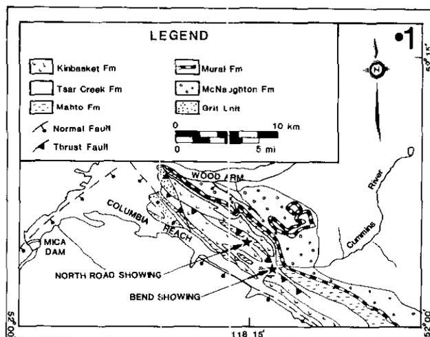
Figure 2-7-1. Regional geology of the Bend property, Cummins River canyon area (after Simony *et al.*, 1980). Geology is shown only for the area surrounding the North Road and Bend showings. The northwest-trending axis of the Porcupine Creek anticlinorium passes approximately through point 1.
