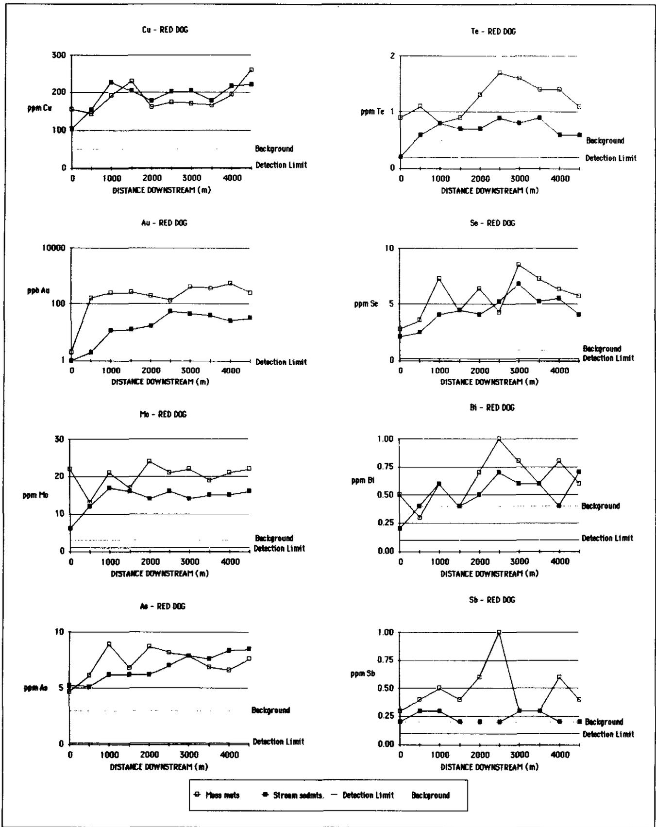
Figure 5-3-5. Downstream dispersion patterns for Au, Mo, Cu, As, Sb, Bi, Se and Te in Red Dog Creek moss-mat and stream sediment samples. Detection limits are from the analytical company's brochure, regional background level determined as described in the text. See Figure 5-3-4 for sample locations.
