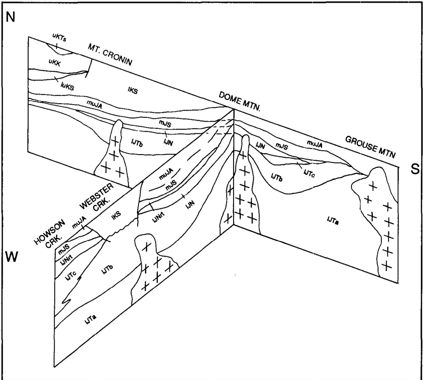
Figure 1-23-3. Stratigraphic fence diagram. See Table 1-23-1 for explanation of symbols.
