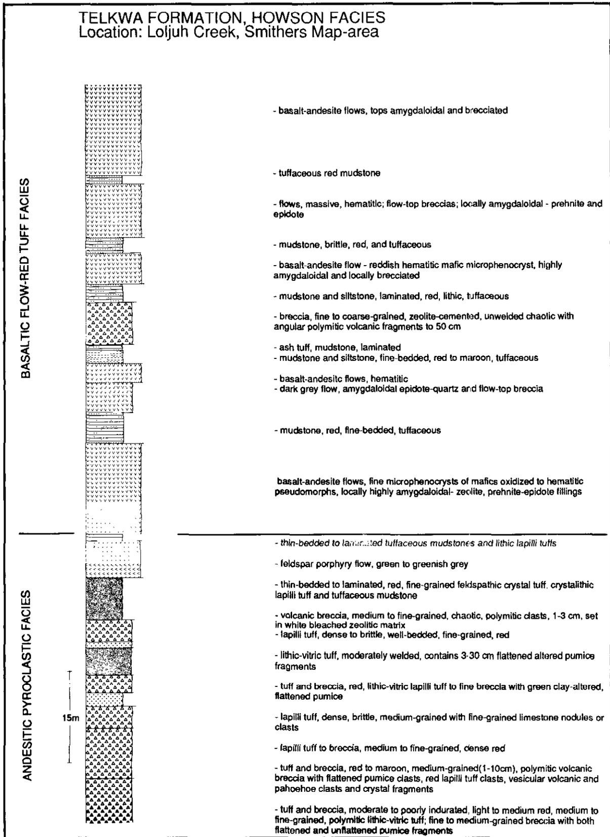
Figure 1-23-5. Stratigraphic section, Lofjuh Creek area (modified after Tipper and Richards, 1976).
