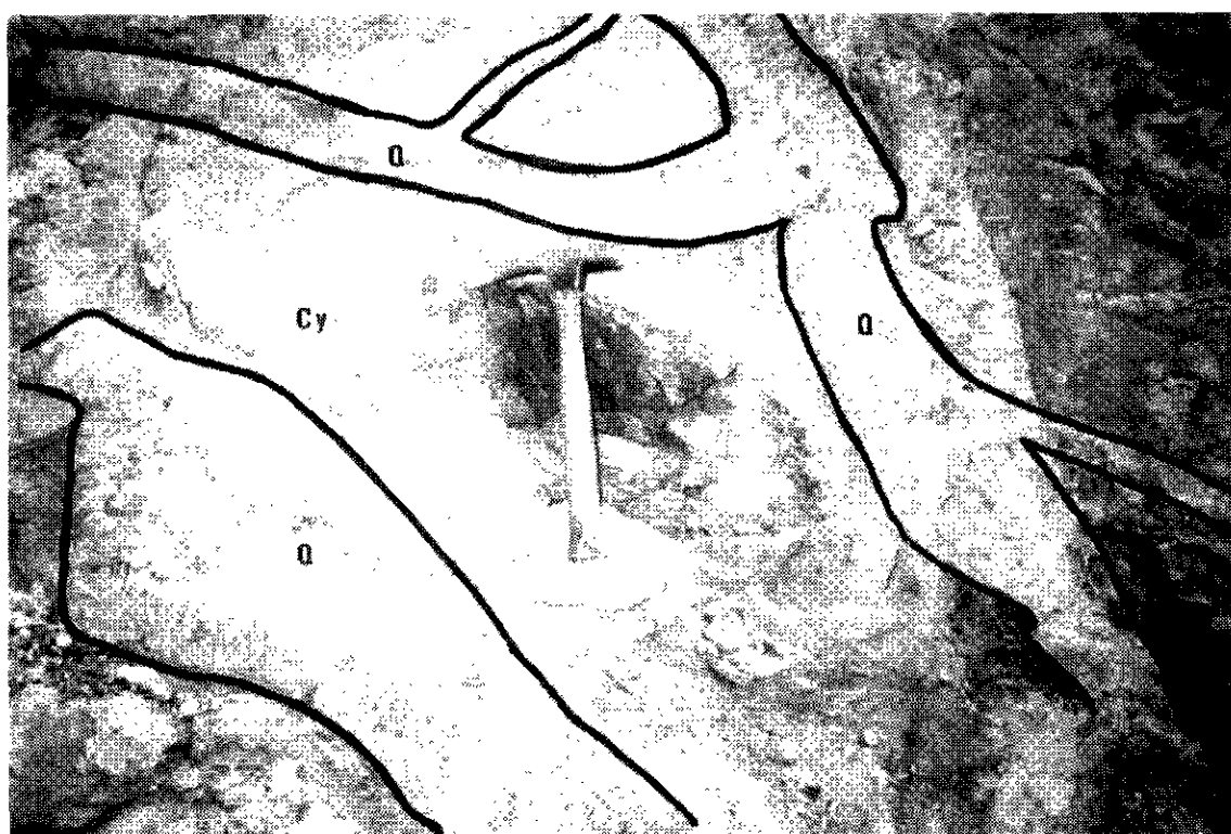
Figure 6. Zone V trench, looking southwest. Note stockwork of auriferous cockscomb quartz-sulphide veins (Q) cutting bleached, clay-altered sandstone (Cy).
