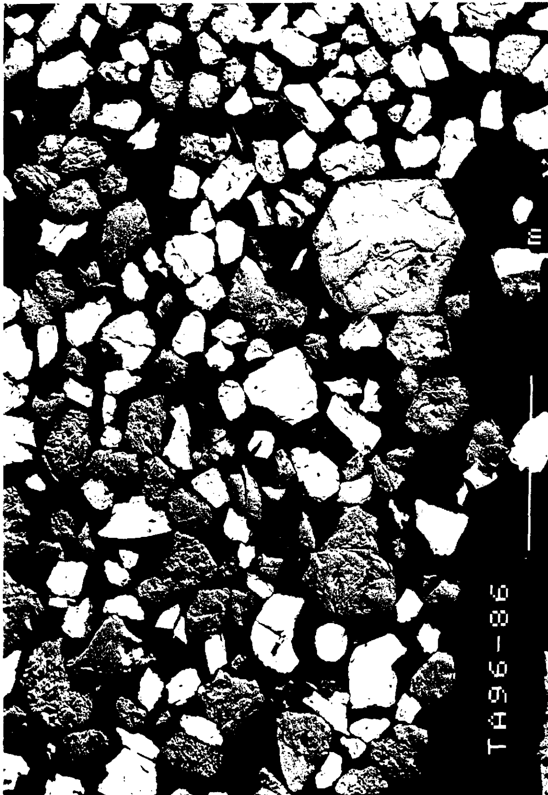
Figure 3: Backscatter microphotograph of the corundum (dark) and rutile (pale) concentrate
