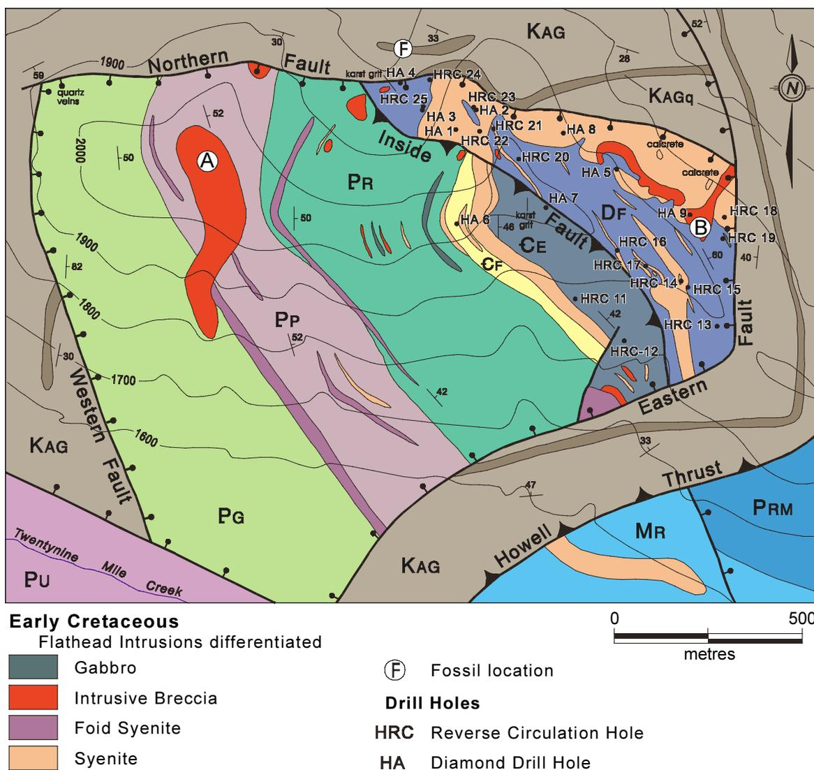
Figure 3. Detailed geology of the Eastern Outlier illustrating syenite and breccia distribution within the Proterozoic and Paleozoic strata (modified from Cameron *et al.* (unpub. map), and Legun (1993)). Drill hole locations are indicated. See Figure 2 for unit descriptions.
