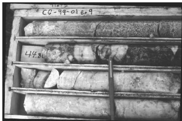
Photo 1 Drill core from Hole CG 99-01, Main vein, Cam-Gloria prospect. The grey and white banded material at 44.8 metres is brecciated quartz and fine grained sulphides at the upper (hangingwall) contact. Coarse-grained white quartz is below and sericitized quartz monzodiorite is above.
