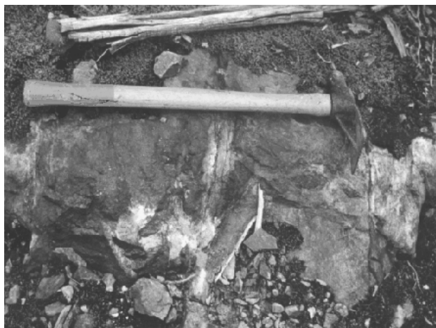
Photo 5. Goldstrike 1 (Bizar) showing. Sheeted quartz-limonite veins cutting micaceous quartzite of the Shuswap metamorphic complex.
