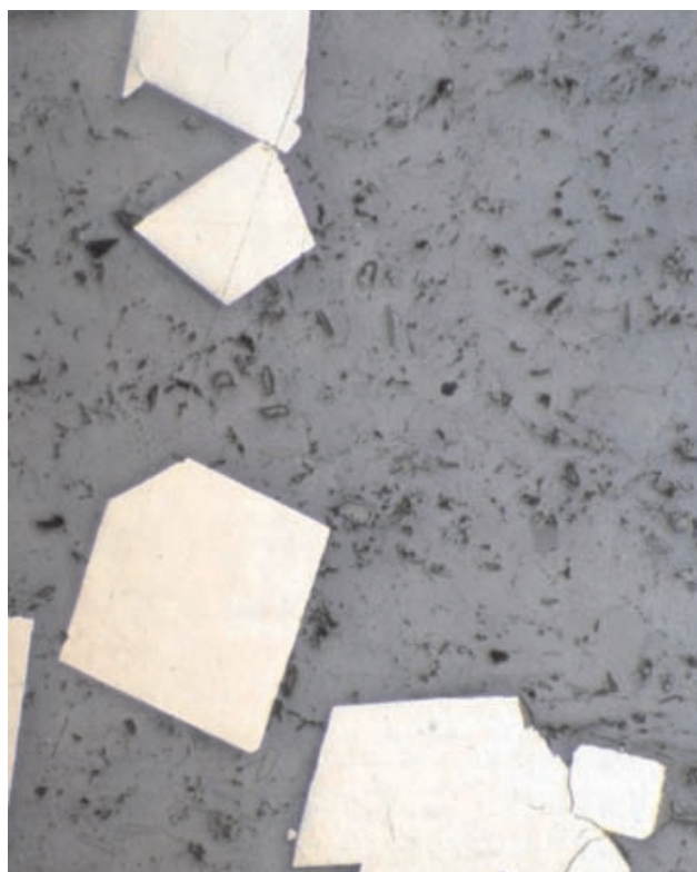
Photo 10. Replacement pyrite ore at the Island Mountain Mine. Coarse auriferous pyrite cubes in a gangue dominated by quartz, lesser sericite and trace rutile. Sample GR-00-86 assaying 49.9 g/t Au. Pyritic float sample taken from the Island Mountain Mine dump. Photomicrograph, reflected light, crossed polars, and long field of view is 2.5 mm.
