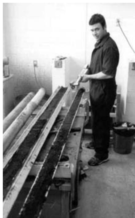
Photo 2. A bone cutter used to cut core tubes in preparation for sampling.
