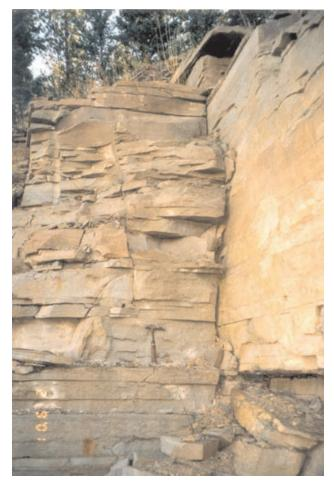
Photo 4. Fracture frequency results in quarrying slabs up to 1 metre in size. Hammer for scale is approximately 30 centimetres.
