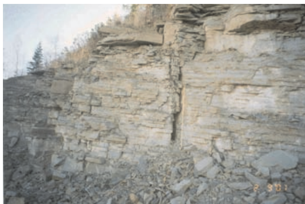
Photo 6. Large patches of white staining, below some bedding planes, indicate soluble salts problem in the sandstone . Seepage comes periodically from many bedding planes after the spring break-up or rainy periods.
