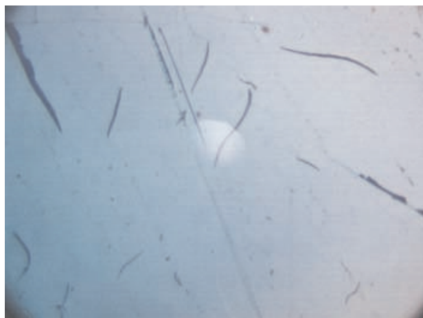
Photo 4. Pseudovitrinite with multiple orientations of slits.
