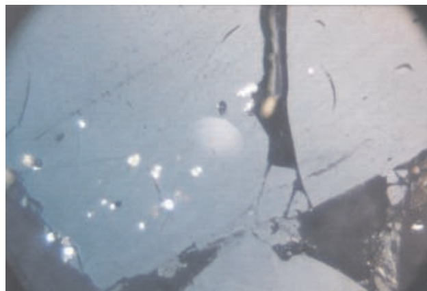
Photo 3. Pyrite in pseudovitrinite grains.
