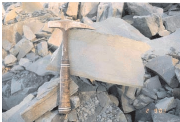
Photo 5. Brown colouration (oxidation) from percolating water along bedding planes.
