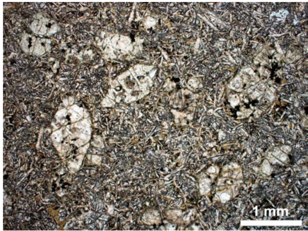
Figure 10. Photomicrograph of high-Mg basalt in a massive sheet flow at the type locality at Keogh Lake. Euhedral to subhedral olivine phenocrysts are set in a groundmass of calcic plagioclase, clinopyroxene and granular opaque oxides. The olivine is completely replaced by talc±chlorite and fine-grained magnetite. Sample 07GNX37-1-1 in plane-polarized transmitted light.
