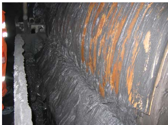
Figure 23: Use of magnetite in coal upgrading process at the Quinsam Coal plant on Vancouver Island (from Simandl and Brûlé (2008).
