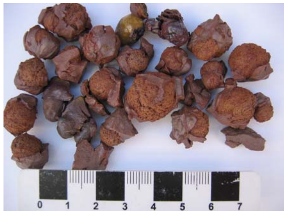
Figure 28: Expanded shale; sample of light weight aggregate produced on experimental scale from expanding shale deposit located on Vancouver Island.
