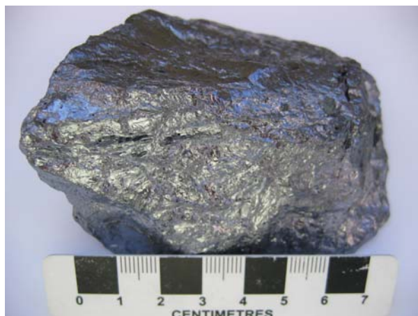
Figure 31: Metallurgical grade silicon produced from British Columbia quartzites. New technology allows such product to be economically upgraded to “solar-grade” silicon.
