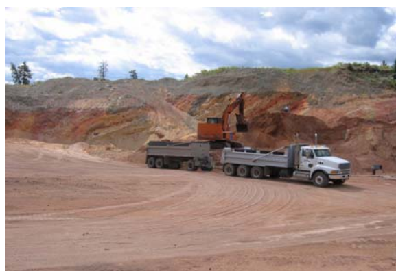
Figure 11: Pacific Bentonite Ltd. ships natural clinker from its Décor deposit (Hat Creek area) to the Lafarge cement plant in Kamloops.
