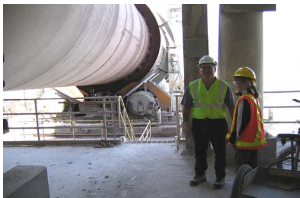
Figure 7: The heart of any Portland cement making facility is a kiln. The Lafarge Canada Inc. cement plant, Richmond.
