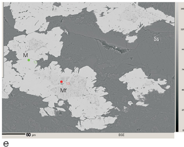
Figure 2e. Scanning electron microprobe (SEM) photomicrograph showing rock polished section, Cr-magnetite grains (Mf) completely surrounded by magnetite (analytical points 12, 13); scale bar 50 µm.
