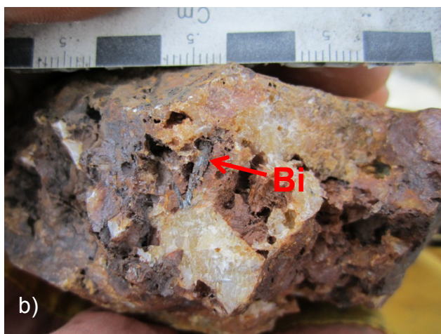
Figure 15. (a) Sheeted, rusty quartz veining in bleached granodiorite. Centimetre-thick veins are typical (beneath hammer). A close-up of the ~10 cm thick vein to the left of the hammer is shown in (b). (b) Vuggy, rusty quartz vein shows angular void outlines of pyrite cubes removed by weathering, and residual bismuthinite crystals (Bi).
