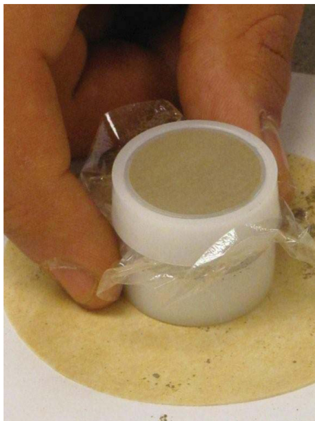
Figure 2. Typical sample cups covered by 4.0 \mu thick polypropylene film.
