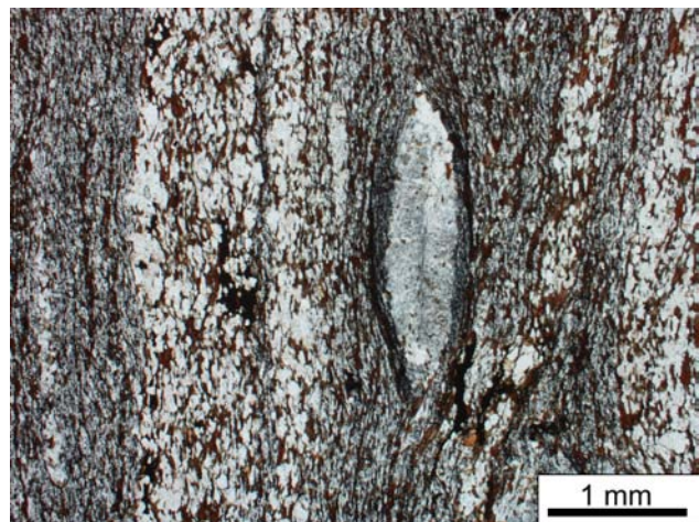
Fig. 6. Biotite-quartz-feldspar gneiss in the hanging wall, 25 metres from the Lonnie complex. Pale grey minerals are quartz and feldspar; biotite is reddish-brown. Darker grey bands are finer-grained, and contain micron-scale opaque minerals. (Plane-polarized light).
