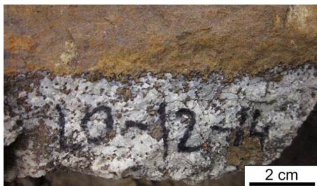
Fig. 13. Aegirine carbonatite–fenite contact. Carbonatite is grey, fenite is rusty brown.
