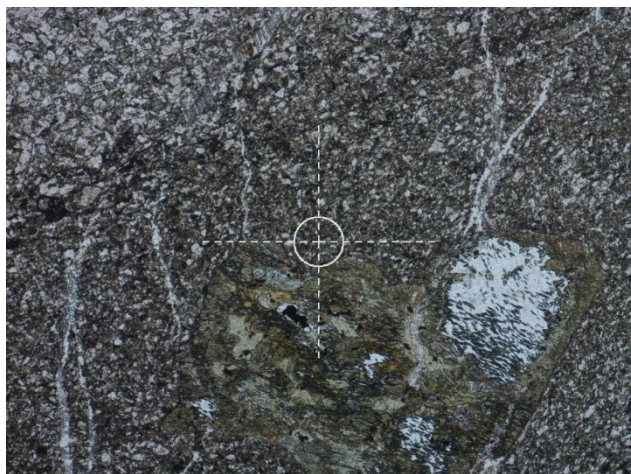
Fig. 8. Photomicrograph of "Cherty tuff" siltstone in plane polarized light. Many silt-sized grains are very angular and crystal shards are common. Bedding, defined by clast size, extends diagonally from middle left to upper right. An outsized clast of foliated, epidote-altered country rock is in the bottom central part of the image. Circle at crosshairs has a radius of 100 \mu .
