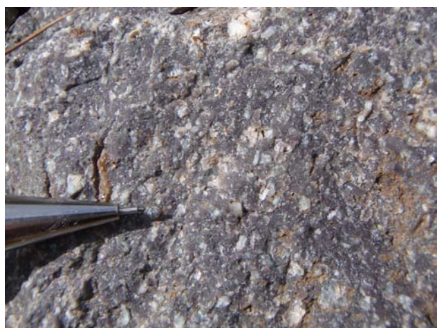
Fig. 6. Quartz-plagioclase-phyric rhyolite, Wineglass assemblage, unit Wv2.
