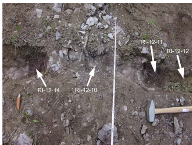
Fig. 6. Central dark purple rock (mineralized zone; sample RI-12-10), adjacent pale purple rock (weakly mineralized contact zone; sample RI-12-11 and RI-12-14), and outer greyish green zone (fresh porphyry; sample RI-12-12). Pocket knife and measuring tape for scale. See Fig. 5 for sample locations.
