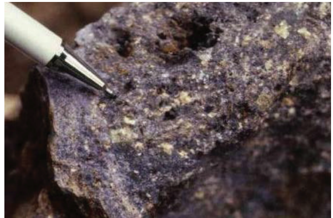
Fig. 1. Bastnäsite (beige rectangular crystals) cemented by fluorite in a sample of sandstone-hosted breccia (numerous small irregularly shaped fragments) from the Gallinas Mountains deposit, New Mexico.
