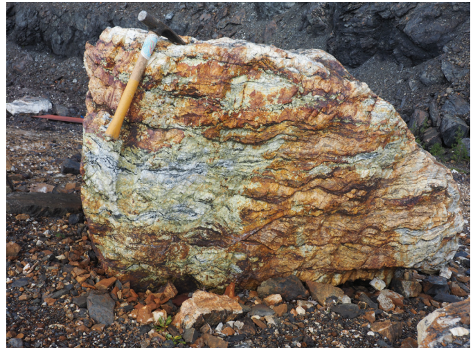
Fig. 23. Sheared quartz with argillite, graphite, and sulphide seams containing gold. Vollaug Vein, Cassiar Gold project (Cassiar Gold Corp.).
