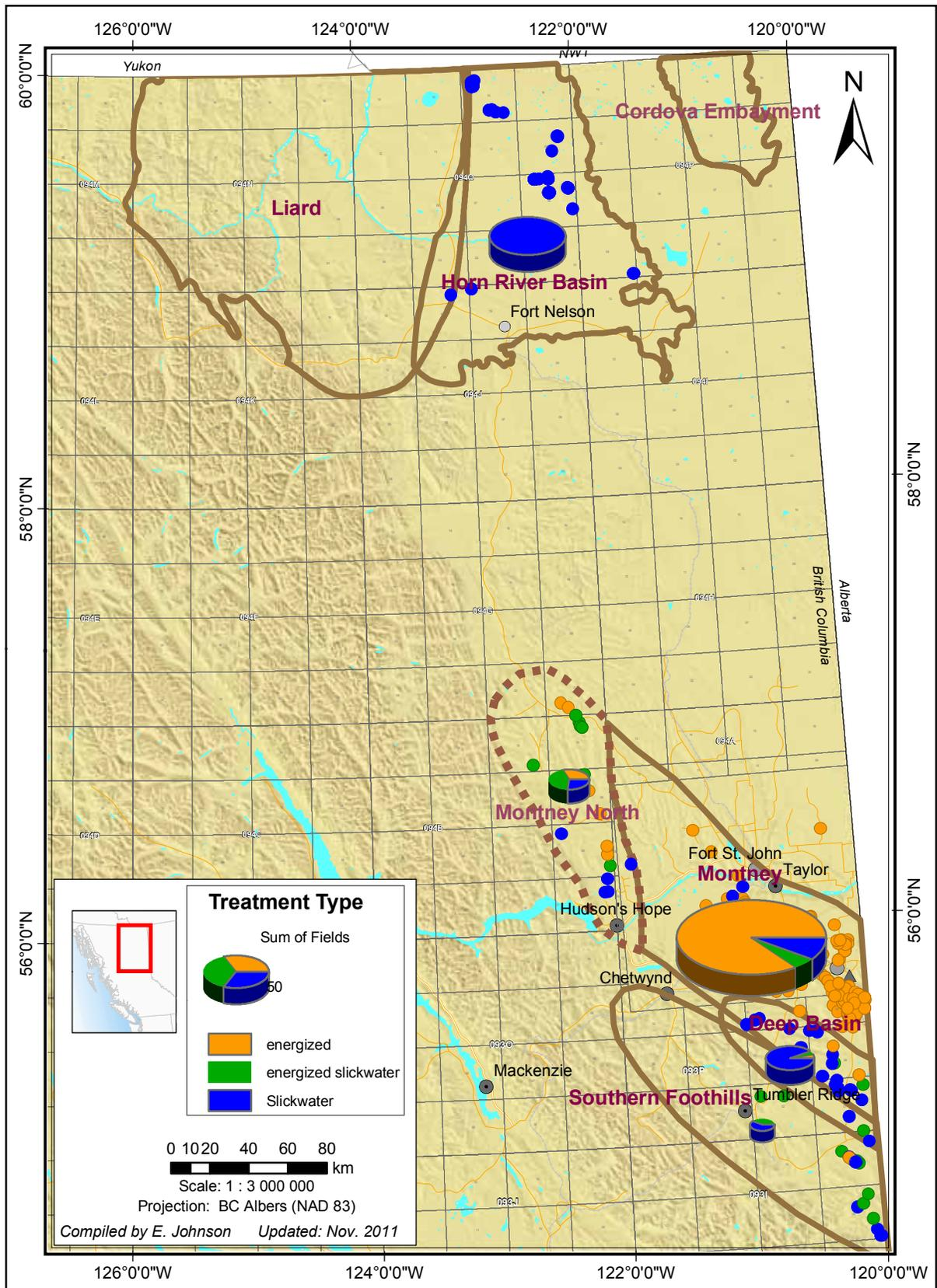
Figure 5. Types of fracture treatments and their distribution across northeast British Columbia. Wells are colour-coded by treatment type and pie charts represent the relative proportion of treatment types for wells a given basin.
