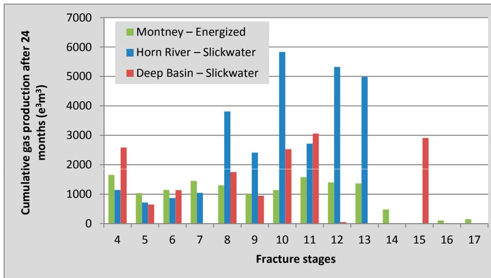
Figure 7. Produced gas as a function of the number of fracture stages per well.
