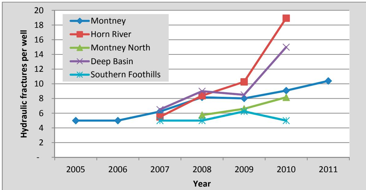
Figure 6. Average number of fracture stages for wells by basin between 2005 and 2010.
