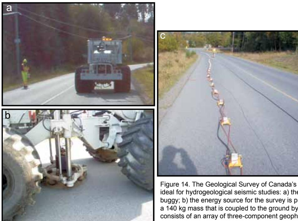
Figure 14. The Geological Survey of Canada's Minivib with land streamer is ideal for hydrogeological seismic studies: a) the vibrator is mounted on a Minivib buggy; b) the energy source for the survey is provided by a vibrator, consisting of a 140 kg mass that is coupled to the ground by hydraulics; c) the land streamer consists of an array of three-component geophones mounted on metal sleds.
