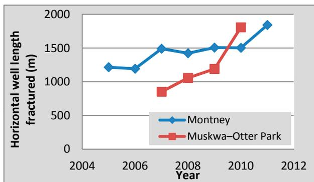
Figure 9. Average horizontal wellbore lengths for two formations between 2005 and 2010.
