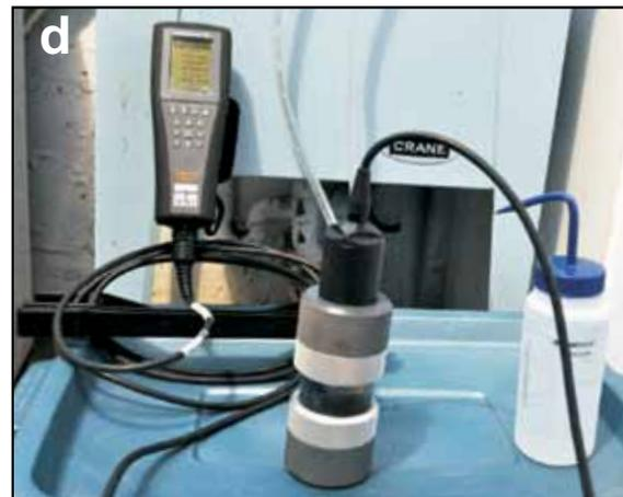
Figure 3. a) Wells included in the water well survey were visited by a contractor and measurements and samples were collected; b) the location and elevation ( $\pm 50$  cm) of each well was determined by precision GPS measurement; c) the static water level was established using a handheld ultrasonic meter; d) a multiparameter flow-through meter was used to determine pH, electrical conductivity, dissolved oxygen and oxidation/reduction potential.
